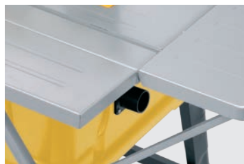
DUST EXTRACTION OUTLET Ø40mm
